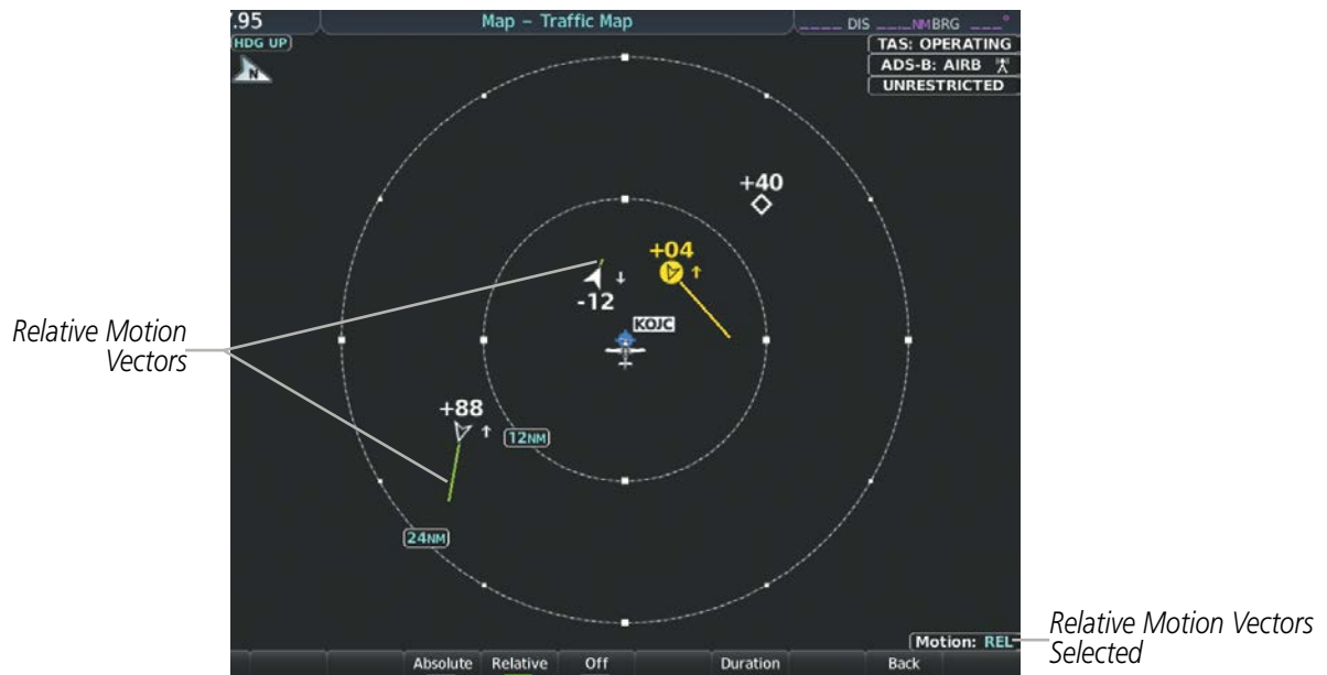
Figure 6-84 'Map - Traffic Map' Page with Relative Motion Vectors Enabled
