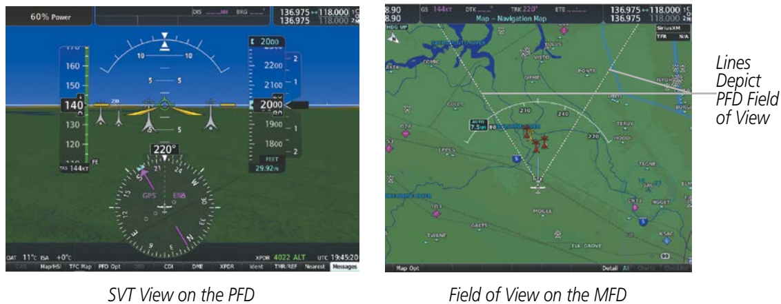
Figure 2-47 PFD and MFD Field of View Comparison
