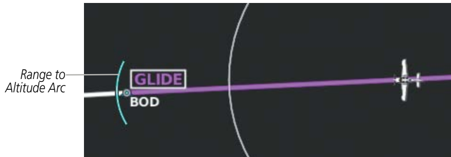
Figure 5-18 Navigation Map - Range to Altitude Arc
