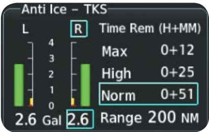
Figure 3-13 Manual Tank Mode (Right tank selected)
