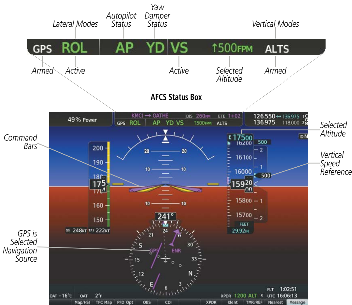
Figure 7-2 PFD AFCS Display
