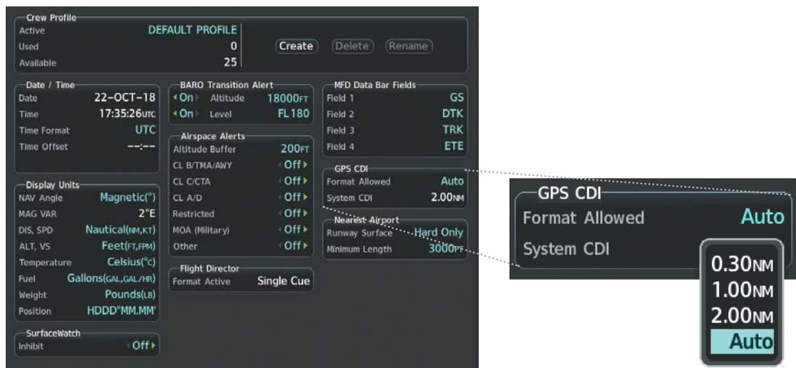
Figure 2-22 GPS CDI Settings (AUX - System Setup Page)
