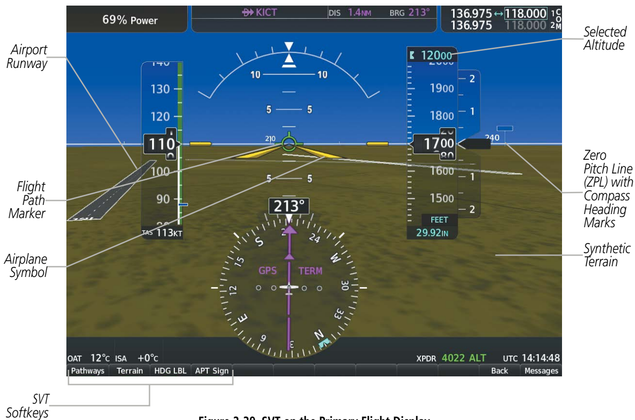
Figure 2-39 SVT on the Primary Flight Display
