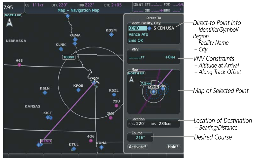
Figure 5-39 'Direct To' Window – MFD
