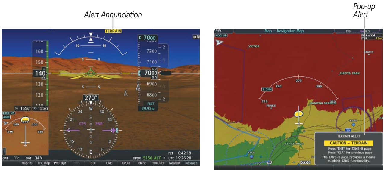
Figure 6-63 TAWS-B Alert Annunciations
