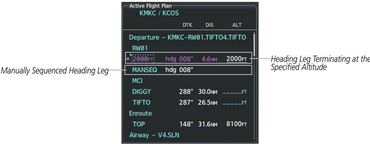
Figure 5-69 Procedure Leg Identifiers
