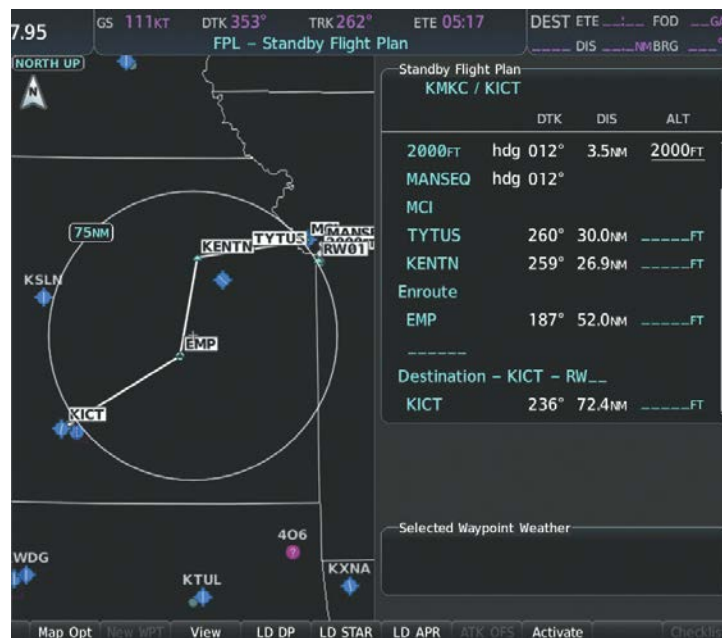
Figure 5-57 'FPL – Standby Flight Plan' Page
