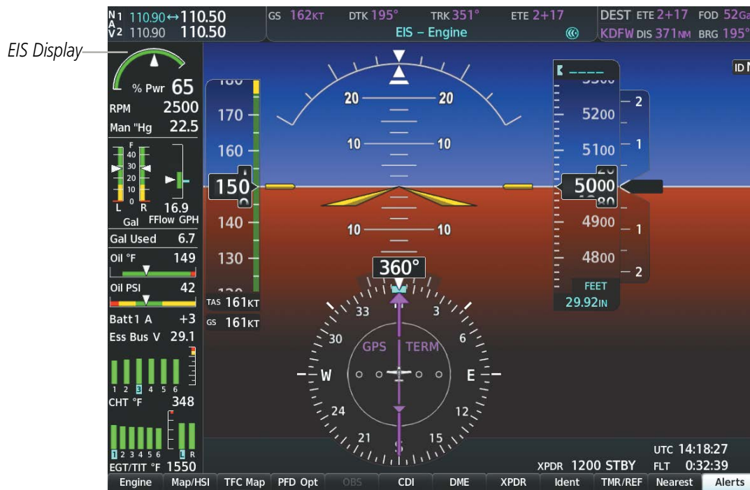
Figure 3-19 Reversionary Mode (SR22T)
