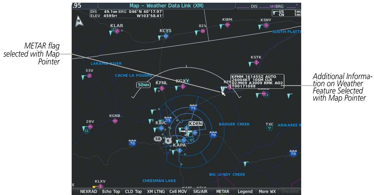
Figure 6-31 METAR Flags on the 'Map - Weather Data Link (XM)' Page
