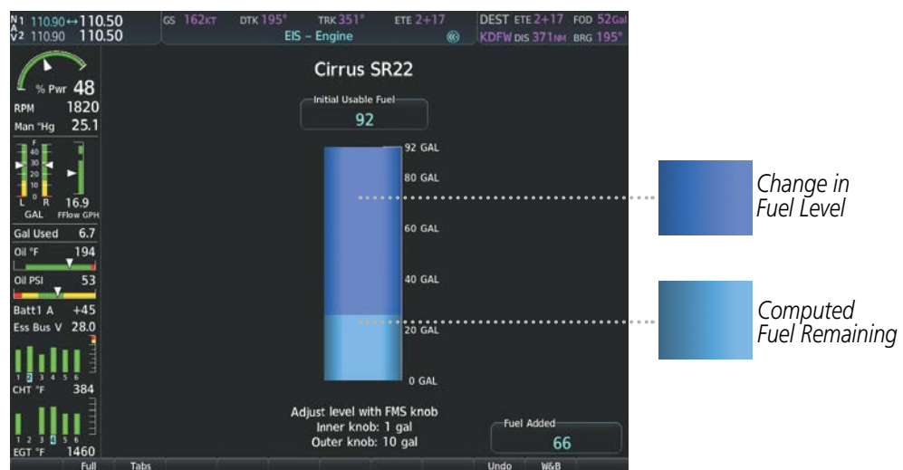
Figure 3-9 Full Fuel (SR22 shown as example) Initial Usable Fuel Page
