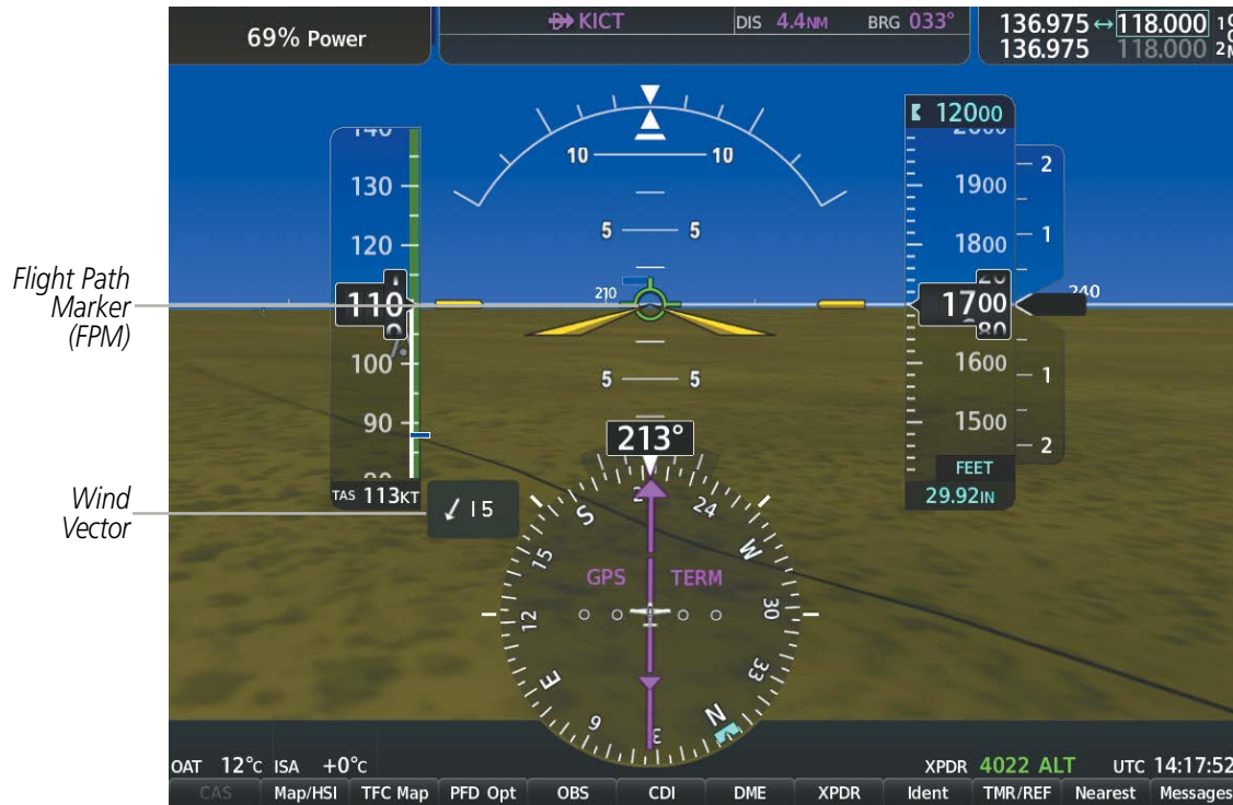
Figure 2-41 Flight Path Marker and Pathways
