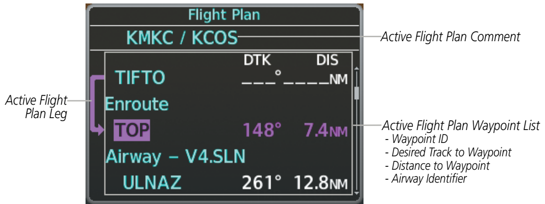
Figure 5-43 'Active Flight Plan' Window on PFD
