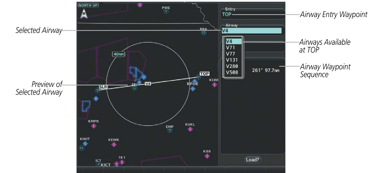
Figure 5-54 Select Airway Page – Selecting Airway
