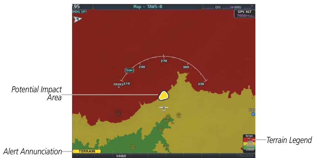
Figure 6-64 TAWS-B Page with Alert Annunciation
