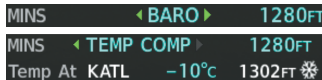
Figure 2-37 BARO and TEMP COMP MDA/DH
