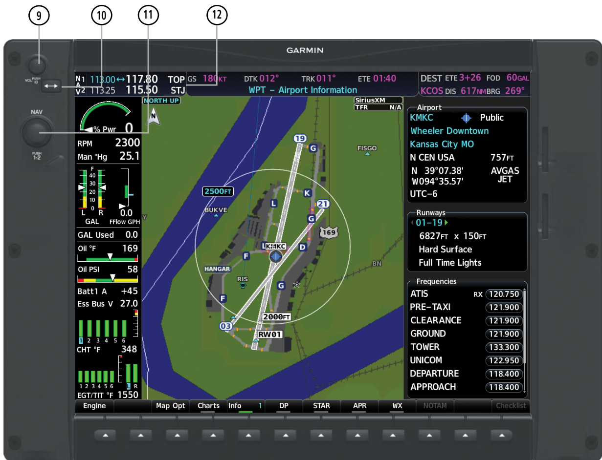
Figure 4-2 MFD Controls and NAV Frequency Tuning Boxes
