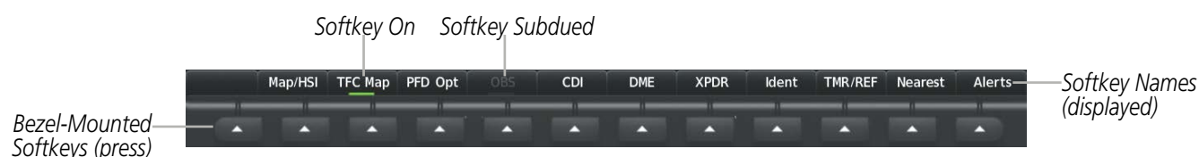
Figure 1-9 Softkeys (First-Level PFD Configuration)
