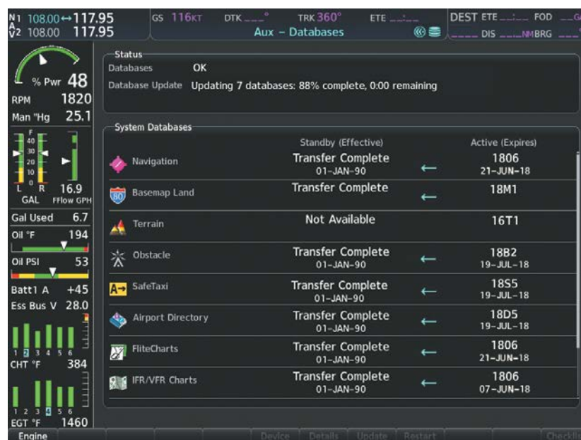
Figure B-10 Device Database Transfer
