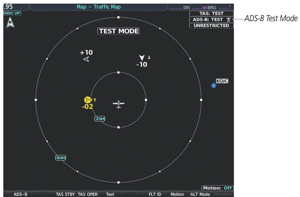
Figure 6-75 System Test in Progress with Test Pattern
