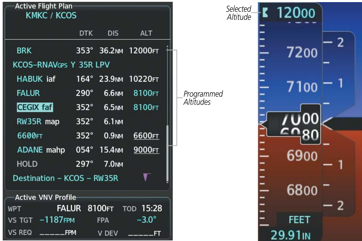
Figure 2-42 Programmed and Selected Altitude
