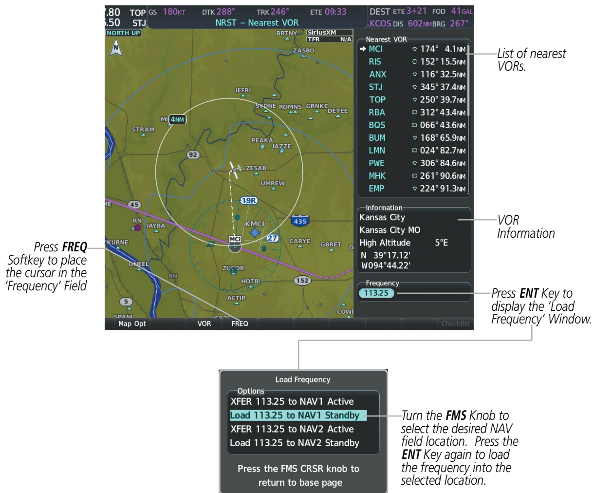
Figure 4-15 Loading the NAV Frequency from the 'NRST – Nearest VOR' Page
