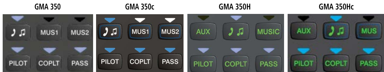
Figure 4-26 Blue-Select Mode (Telephone/Entertainment Distribution)
