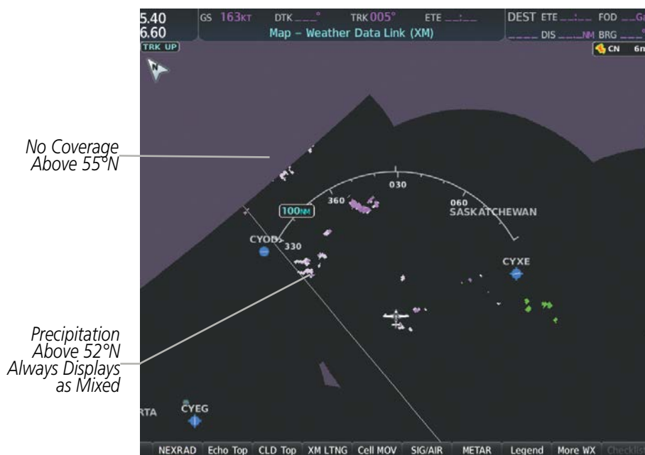
Figure 6-12 NEXRAD Weather Product on the 'Map - Weather Data Link (XM)' Page - Canada
