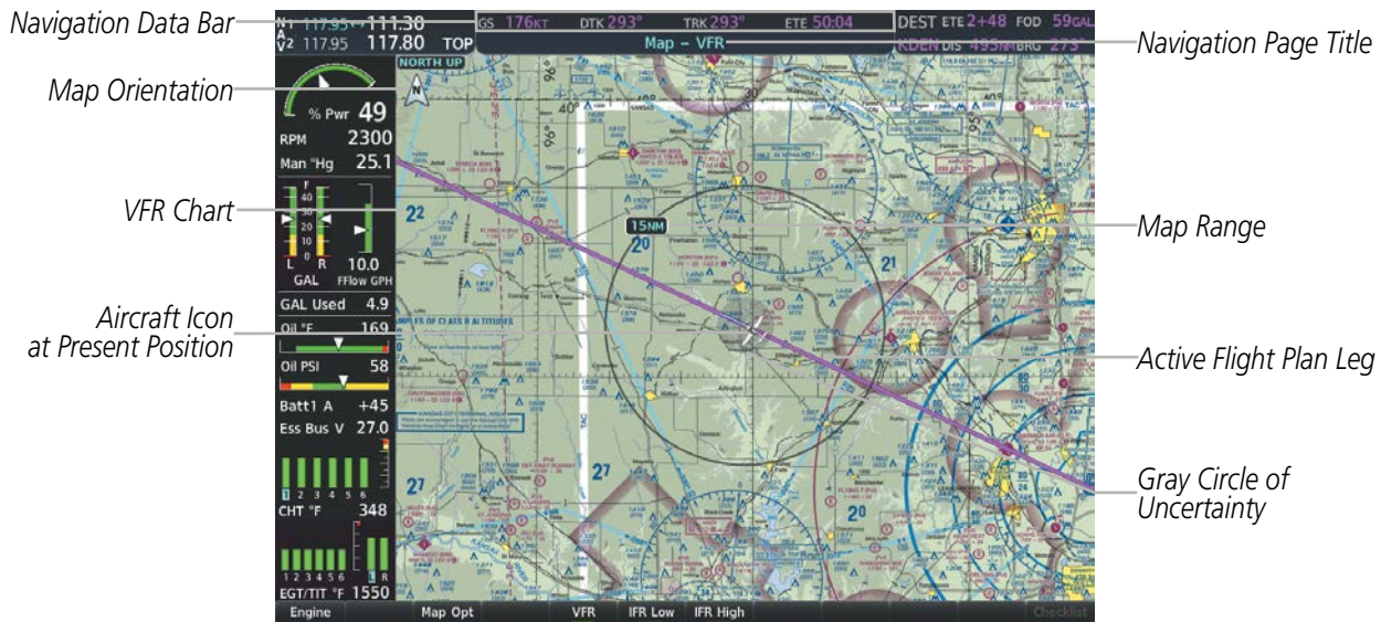
Figure 8-23 GPS Navigation Information on the VFR Chart
