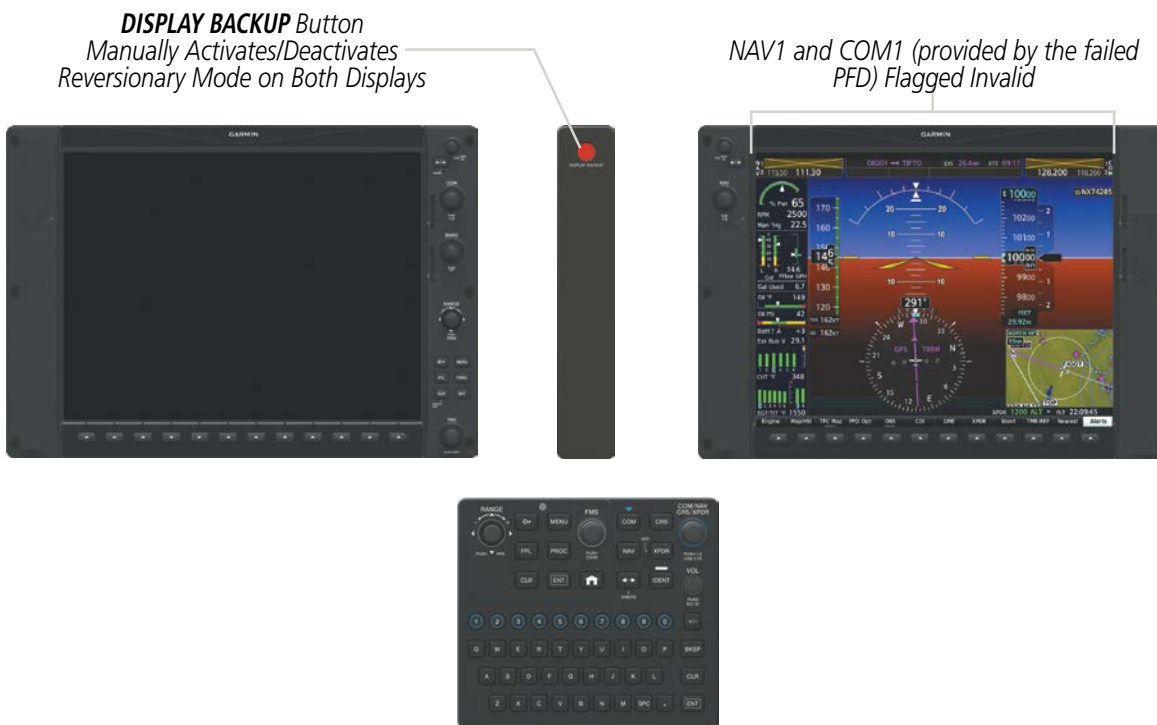
Figure 1-6 Reversionary Mode
