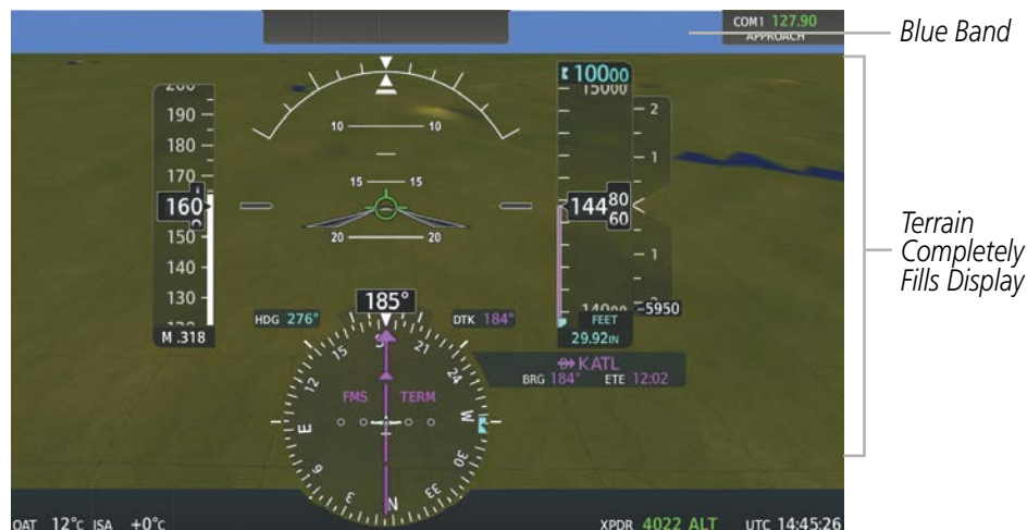
Figure 2-50 Blue Sky Bar with Full Display Terrain
