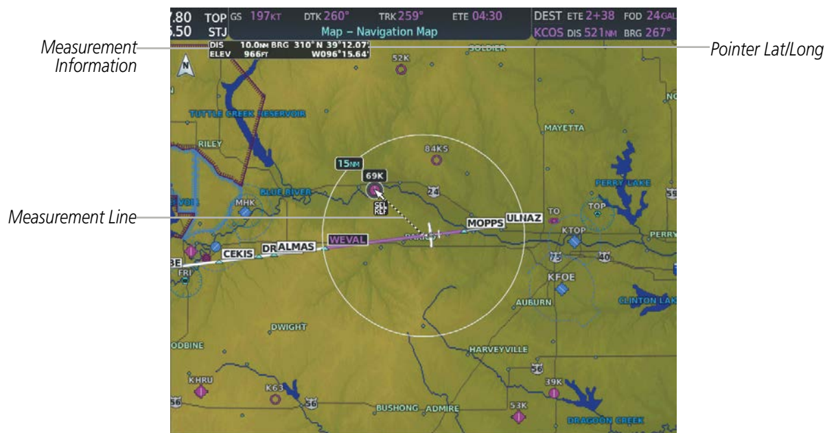
Figure 5-12 Navigation Map - Measuring Bearing and Distance
