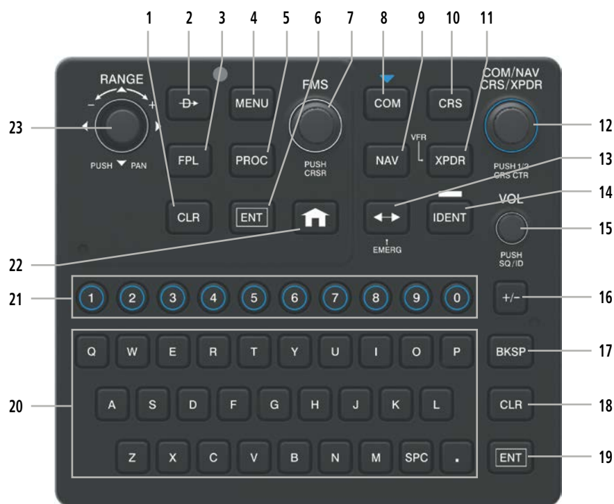
Figure 1-3 Display Controller (GCU 479)
