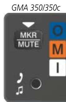
Figure 4-16 Marker Beacon Keys and Annunciator Lights
