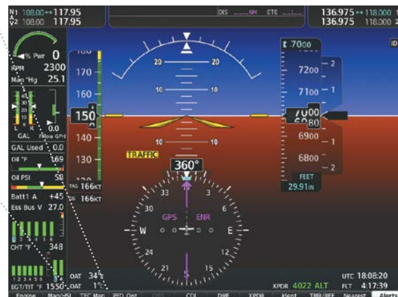
Figure 2-28 Outside Air Temperature
